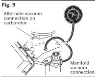
On many systems, little or no vacuum is applied to the distributor at idle; as the throttle is opened wider (engine RPM increases), the vacuum gradually increases. The manifold vacuum drops when the engine is accelerated in proportion to the amount of throttle advance. The gauge should read
