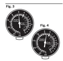
on non-emission controlled engines (pre-1968) indicates correct engine vacuum. Readings may vary considerably on different engines. but should not fall below these minimums. (See manufacturer's specifications).
