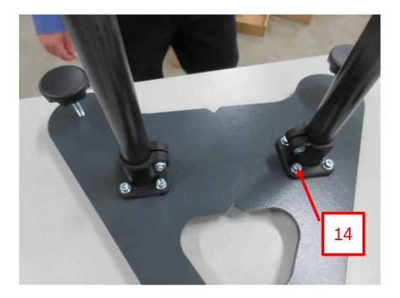
14. Repeat the process of installing the second Guide Tube on the Base Plate.
