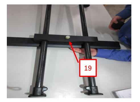
19. Install Tool Holder top half onto bottom half.
