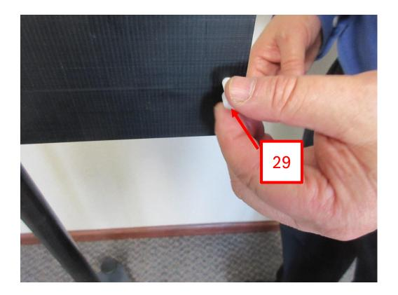
29. Install plastic screws in the Tool Holder at each end to prevent Prismatic Reflector from sliding off.
