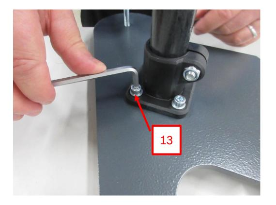
13. Install hex cap screws & tighten to 6nm.
