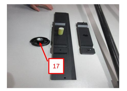
17. Remove Knurled Screw & separate Tool Holder halves.
