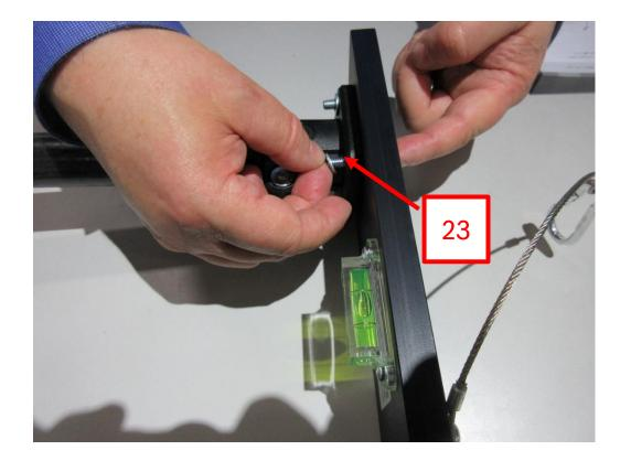
23. Install the counter sunk bolts through Line Laser Mount & Guide Tube, install washers & hex nuts.
