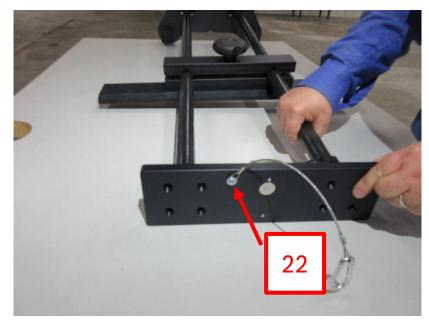
22. Attach Line Laser Mount to Guide Tubes, Arrester Cable & Spirit Level, these should point toward the Base Plate triangle.
