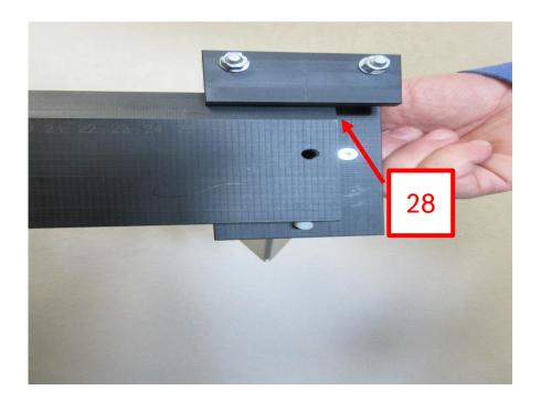
28. Slide Prismatic Reflector onto the Tool Holder.
