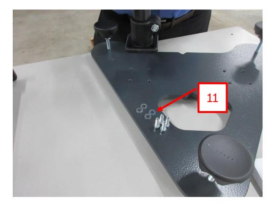
11. Place Guide Tube on to Base Plate, locate Hex Screws & Washers.
