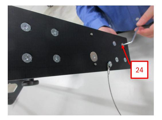
24. Tighten counter sunk bolt hex nuts to 6nm.
