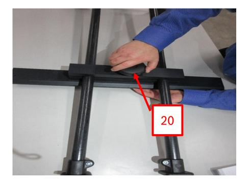
20. Install Knurled Screw and tighten.
