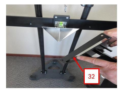
32. Install Laser Range Finder Mount over the top of the Prismatic Reflector.
