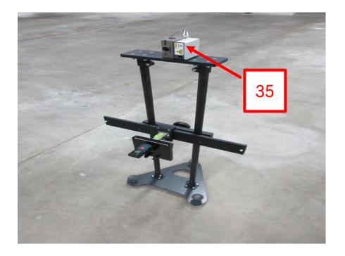
35. Install the Line Laser on the Line Laser Mount & install the Arrester Cable to secure the Line Laser.
