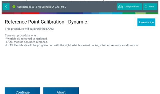
Next, we will give vehicle specific instructions about vehicle set up procedures that must be completed to run the test:
