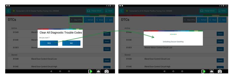
**Special Tests** on FCA SGW enabled vehicles also requires internet connection. Ensure ADS device is connected to the internet, and open up desired a Special Test to begin the process:
