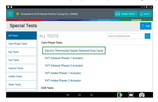
Tap on a Special Test, wait for SGW to be unlocked and the test will be made available:
