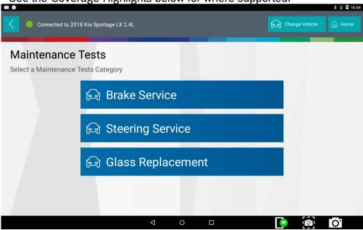
• Tapping on the Glass Replacement selection brings up all available "Dynamic" tests that are available for the selected vehicle. Tap the test to launch the desired calibration test:
