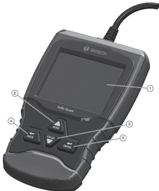
1. LCD display (color, backlit, QVGA resolution)
