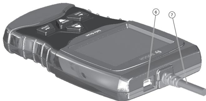
6. USB port provides USB connection for the computer.
