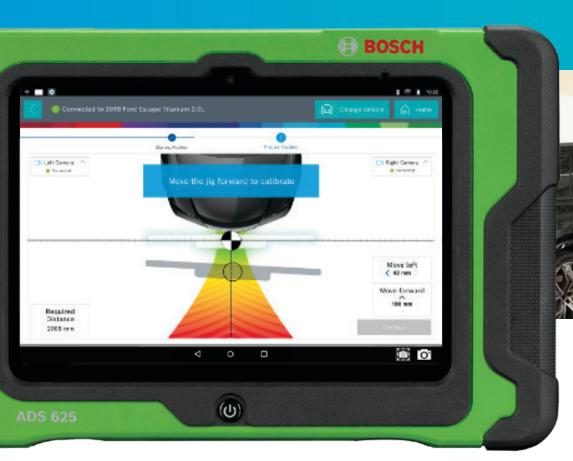
The DAS 3000 utilizes the ADAS workflow process on the ADS 625 to walk you through the calibration, step-by-step, for every vehicle.
