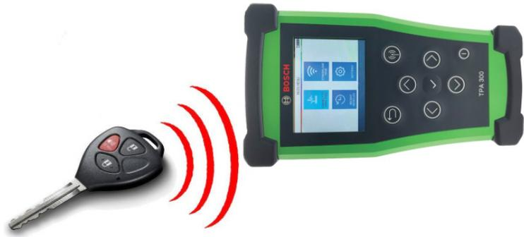
This function tests the strength of the RF signal of the key fob.
