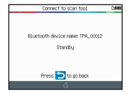
**Step 1:** Put the TPA 300 into "Connect to scan tool" mode.
