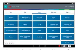
**Step 2:** Select the make, model, year of the vehicle from the scan tool menu, using Auto Id or Manual method. Then choose maintenance test, or special tests, then choose TPMS Registration.
