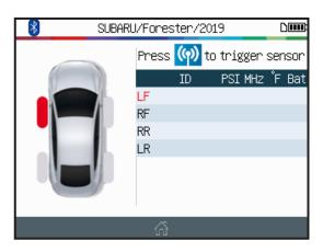
At this stage, you have to read all the TPMS sensor IDs using the TPA 300 tool, exactly the same way you do in Standalone mode. If you are not already familiar with this procedure, see the dedicated section in this user manual.
