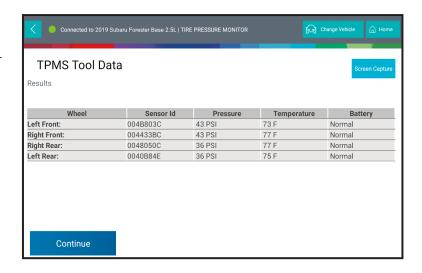
The Bosch scan tool will confirm the correct recording of the new sensors' IDs into the vehicle ECU.
