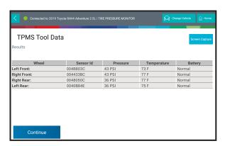
**Step 4:** Follow the scan tool on-screen procedure to register the sensors ID's into the vehicle's ECU.
